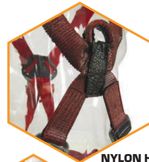
NYLON HARNESS EXPOSED TO ARC FLASH
