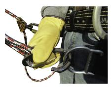
The gate of the locking carabiner is opened by sliding it toward the nose of the hook and twisting it 90 degrees. Simply place the carabiners in the D-Rings of your tool belt with the gate facing out away from your body.
