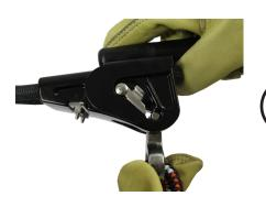
Slide the connector key past the latch gate locking it in place.
