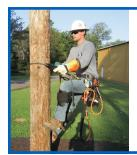
The Patriot™ is lightweight and its ergonomic design reduces stress on the upper body by allowing classically proper climbing technique—proper spacing from the pole, knees out and hips back.
