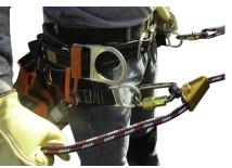
The tail or free end of the line should be to the outside for easier adjustment of the inner Red/White/Blue line.
