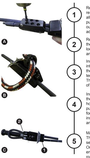
Remove the old rope by removing all of the screws from all 4 sides of the rope clamp and pulling the pieces of the rope out of the connector body and adjustor body. [A]
