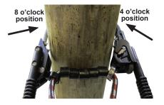
Continue step 1 until the spikes are at the 8-4 o'clock position on the pole and the nylon rollers are touching the pole.
