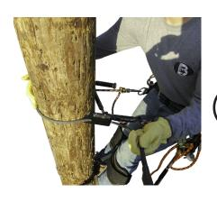
When climbing, the black rope will need to be shortened as the pole tapers. This is done by grabbing the end of the line, placing your right hand on the pole and leaning in slightly to remove the tension on the line. At the same time, push the end of the black line away from the body at 45 degree angle. The angle of the push is critical for easy adjustment. If the angle is too steep or too shallow, the line will not slide through the adjustor smoothly.
